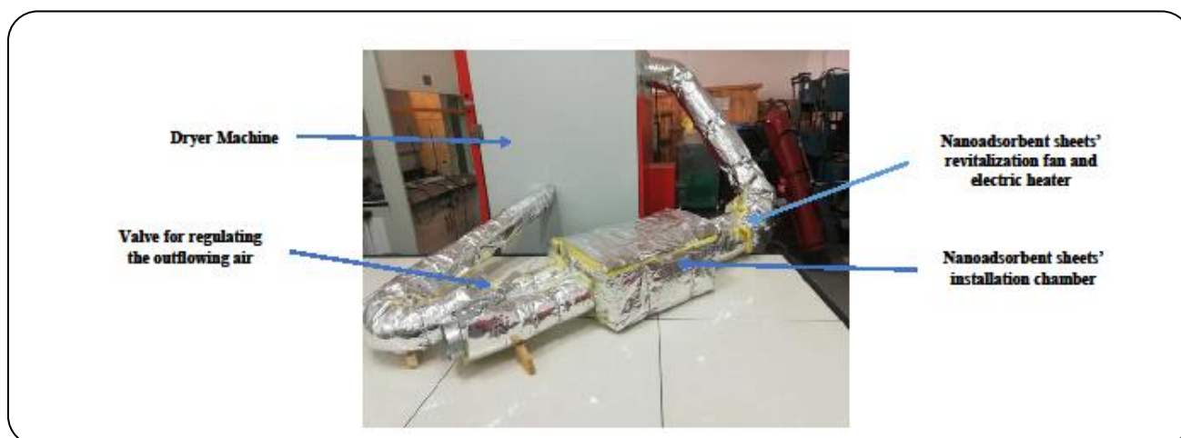
Fig. 1: The photo of the chamber wherein the nano adsorbent sheets and other equipment are installed and the method of their connections to the dryer
