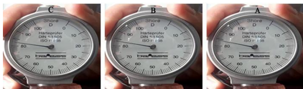
Fig. 9. Shore D test of coating (A= fresh hydrophobic \text{TiO}_2 coating, B= after 24 h salt spray, C= after 48 h salt spray)
