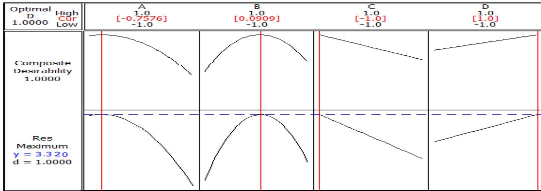
Fig. 5: Parameter optimization of pH (A), temperature (B), the substrate (C), and time (D) affecting hydrogen production;
