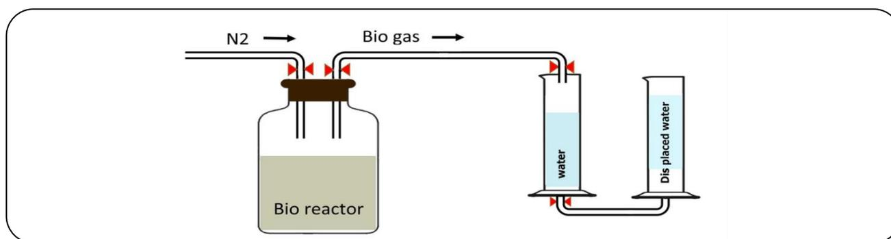
**Fig. 1: Schematic illustration of the designed bio-reactor.**
