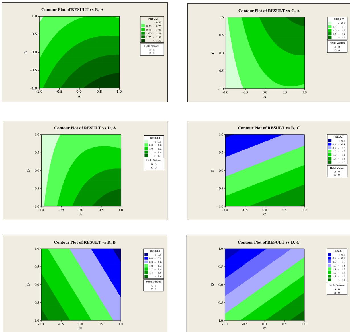
Fig. 6: contour diagrams for pH (A), temperature (B), the substrate (C), and time (D) affecting hydrogen production.
