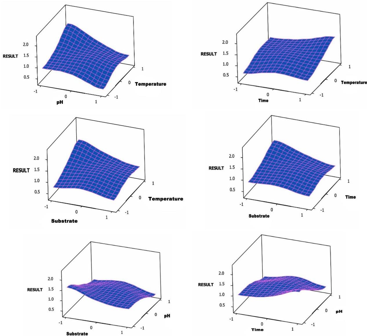
Fig. 4: Effects of temperature (A), pH (B), time (C) and substrate (D) parameters on bio-hydrogen production (molH<sub>2</sub>/mol glucose).
