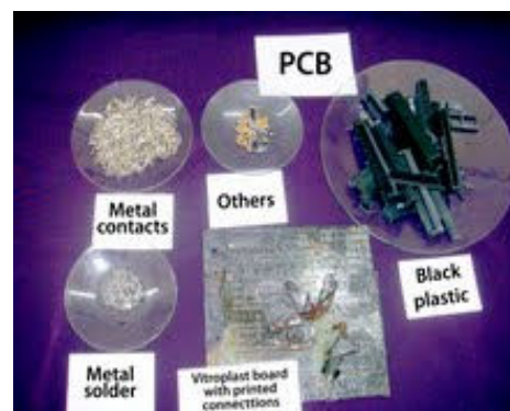
Fig. 3: Parts of PCB after manual disassembling.
