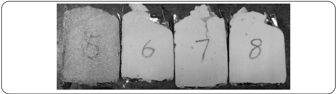
Fig. 9: Longitudinal sections of foams with different surfactant loadings
