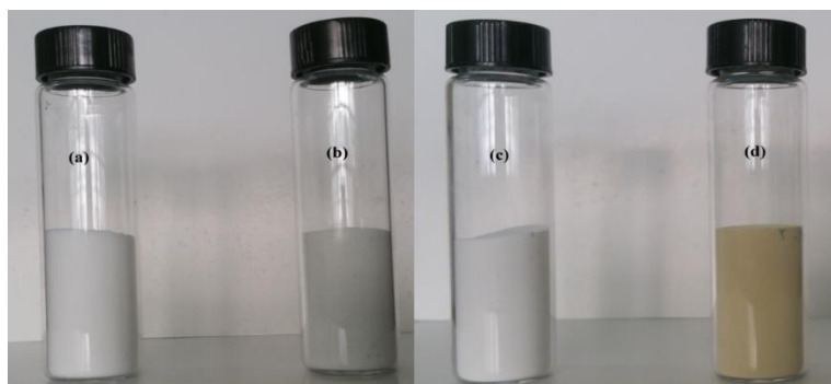
Fig. 3: The physical change (color) onto the carriers before and after the experimental run, (a) SiO 2 before experiment, (b) SiO 2 after 1 st experimental run, (c) Al 2 O 3 before experiment and (d) Al 2 O 3 after 1 st experimental run.
