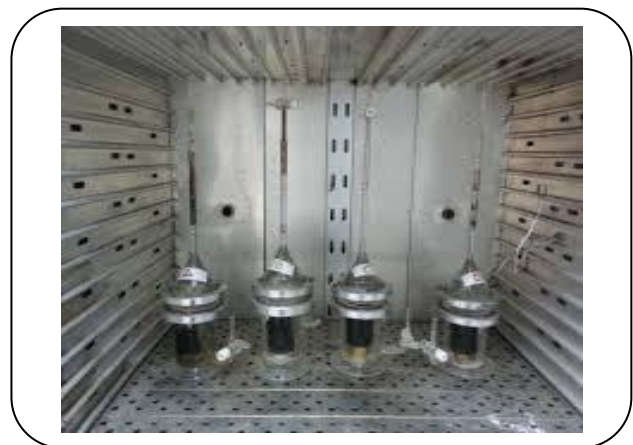
Fig. 4: Experimental Amott cells set up in the oven.
