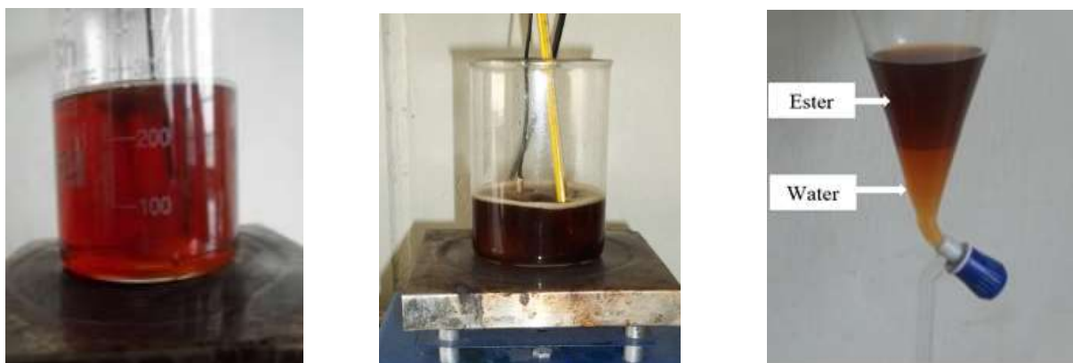
Fig. 4: (a) CD oil, (b) CD oil during esterification, (c) Phase separation after esterification.
