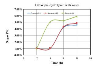
Fig. 2: The percent conversion of OISW pretreated with water at three different ratios.
