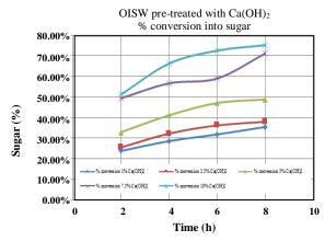
Fig. 4: The percent of glucose obtained from the hydrolysis of OISW samples pre-treated with various concentrations of  $Ca(OH)_2$  solution.
