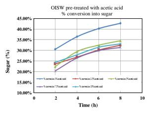
Fig. 5: The percent conversion of OISW pre-hydrolyzed with acetic acid.
