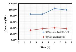
Fig. 7: The percent of glucose obtained from hydrolysis of OISW under an air pressure of 10 psi.
