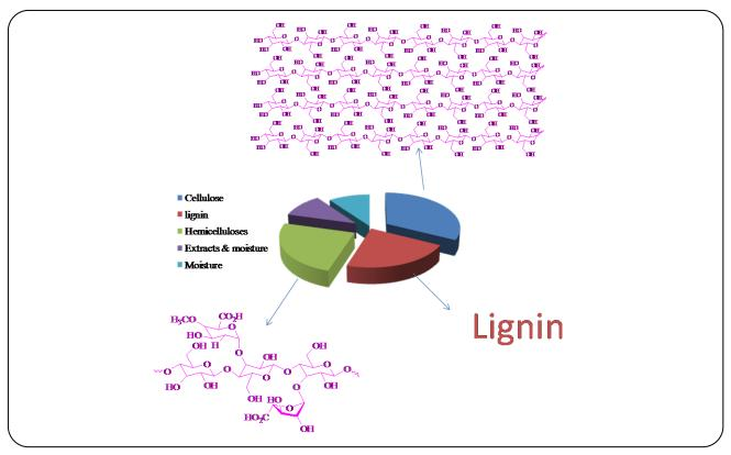
Fig. 1: components of OISW.
