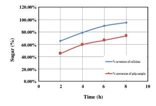
Fig. 6: Hydrolysis results of pulp and cellulose extracted from OISW.
