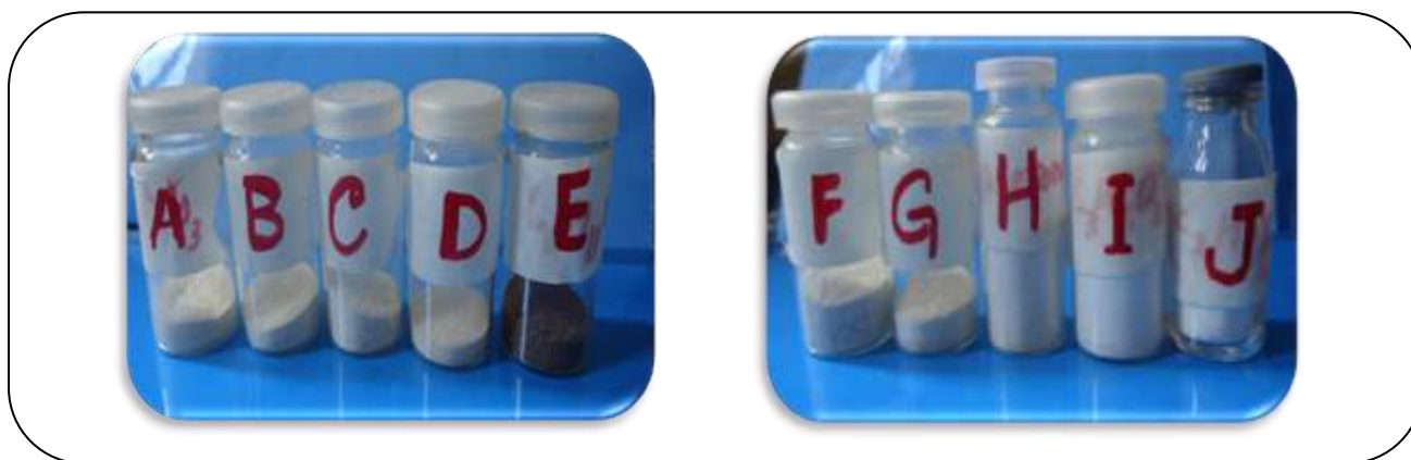
Fig. 1: Synthesized samples of titanium dioxide nanoparticles A (ammonia), B (methanol), C (n-Hexane), D (distilled water), E (diethanol ammine), F (acetic acid), G (acetonitrile), H (acetone), I (propionic acid), J (diethyl ether).
