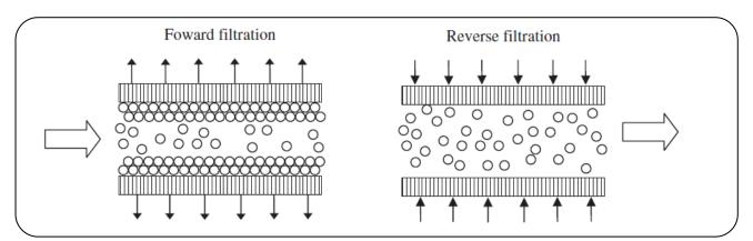
Fig. 5: Schematic representation of forward and reveres filtrations [123].
