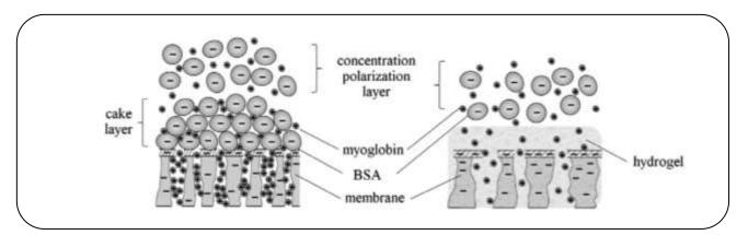
Fig. 10: Comparison between modified and unmodified membrane for separating BSA and myoglobin at pH=6. At this pH, myoglobin is positively charged and BSA and membrane have negative charge [87].
