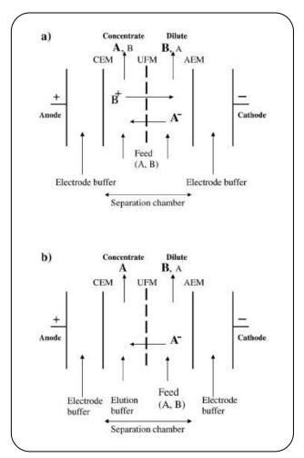
Fig. 7: a) Electrophoretic membrane contactor: separation mode; UFM: ultrafiltration membrane; AEM: anion-exchange membrane; CEM: cation exchange membrane. b) electrophoretic membrane contactor: elution mode [22].
