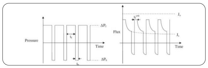
Fig. 6: The trends of pressure and flux within back-pulsing [123].
