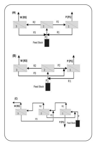
*Fig. 9: Different configurations used for cascade ultrafiltration. A) ideal like configuration, B) adapted configuration and C) counter-current configuration [135].*
