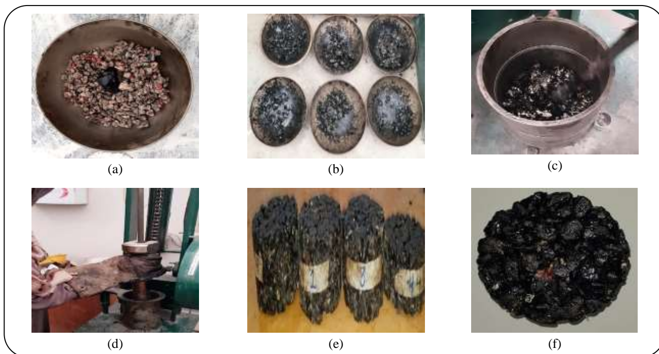
Fig. 5: (a) Sample before being mixed with bitumen (b) Heated samples from oven (c) Sample being added in Marshall Mold (d) Rammer being attached to the Compaction Pedestal (e) Molded samples (f) Top view of the sample
