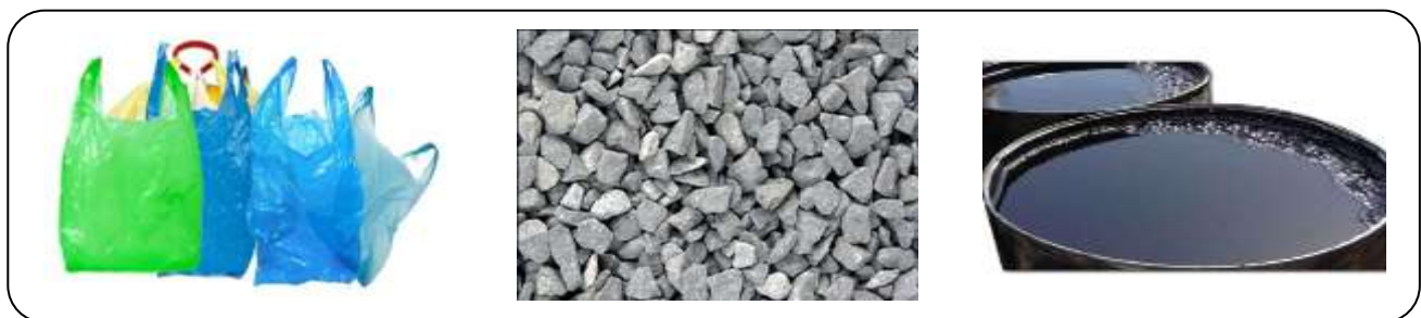
Fig. 2. Raw materials for PCA preparation.
