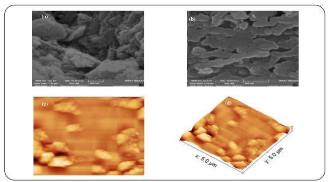
Fig. 2. SEM images of (a) bulk  $g-C_3N_4$  and (b)  $g-C_3N_4$  nanosheet, and (c) AFM image of  $g-C_3N_4$  nanosheet.
