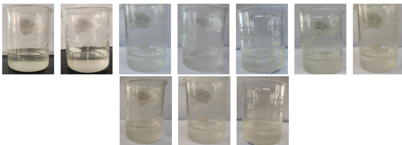
Fig. 9: Photos of fresh water containing Acrylic + 8% Zn_3(PO_4)_2 + 5mM AgNPs coated mild steel exposed for 30 days.
