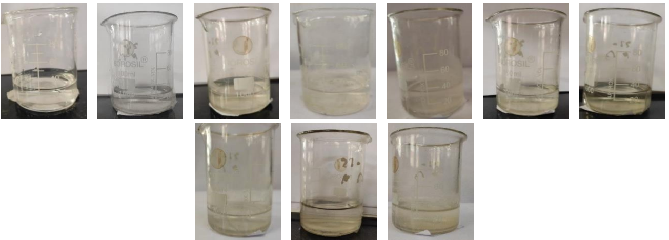
Fig. 11: The photos of demineralised water containing Acrylic coated mild steel exposed for 30 days.
