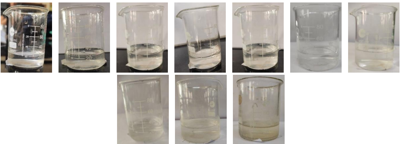
Fig. 12: The photos of demineralized water containing Acrylic + 8% Zn_3(PO_4)_2 coated mild steel for 30 days.
