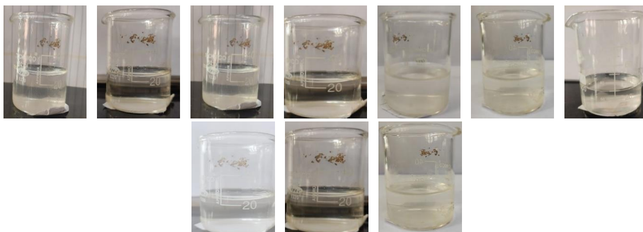
Fig. 8: The photos of fresh water containing Acrylic + 8% Zn_3(PO_4)_2 coated mild steel for 30 days.
