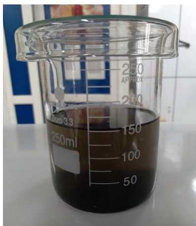
Fig. 4: GO-SiO 2 nanocomposite suspension
