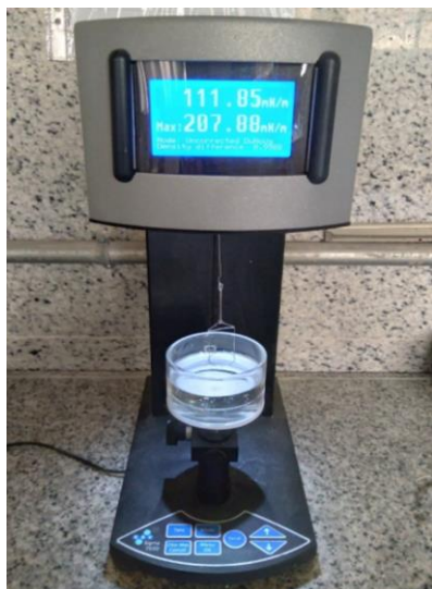
Fig. 6: Sigma 703D force tensiometer device employed to measure IFT values
