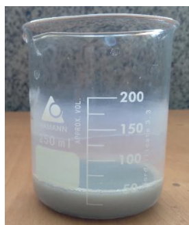
Fig. 16: (2500 ppm GO-SiO 2 -TiO 2 -500 ppm SDS) Hybrid nanofluid
