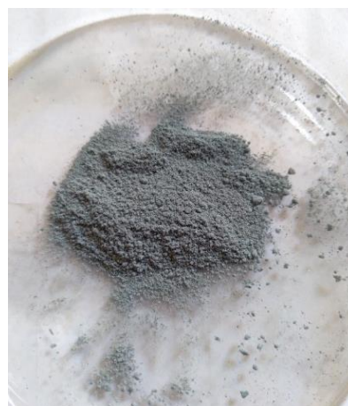
Fig. 5: GO-SiO 2 -TiO 2 nanocomposite powde
