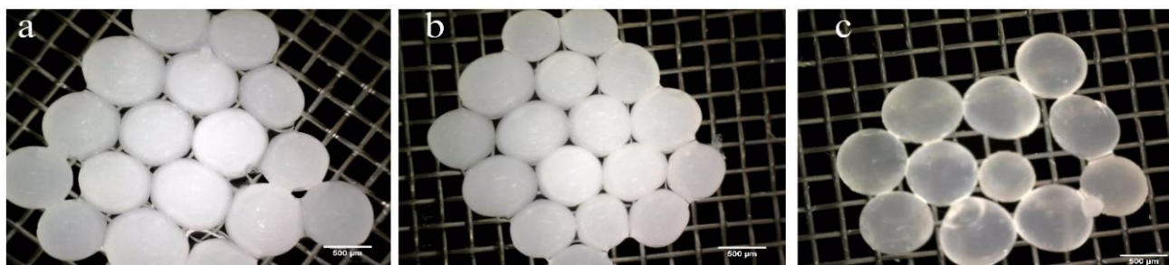
Fig. 2: Morphology of alginate hydrogel beads containing linseed and black seed oil (a,b) and empty hydrogel as control sample (c)
