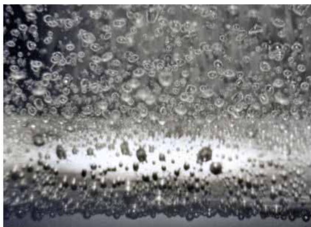
Fig. 11: The appearance of heat transfer surface during pool boiling of acetone ( q=127 kW/sqm).
