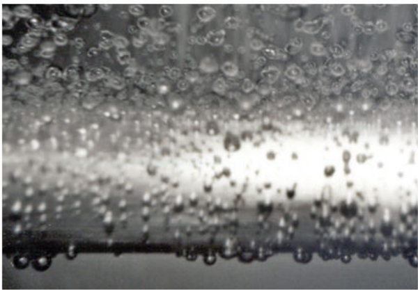
Fig. 19: The appearance of heat transfer surface during pool boiling of water/acetone ( q=147 kW/sqm; x , acetone=0.5 mole).
