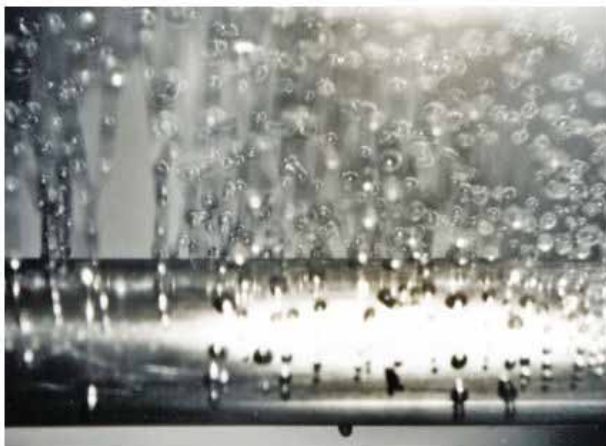
Fig. 10: The appearance of heat transfer surface during pool boiling of acetone ( q=48 kW/sqm).
