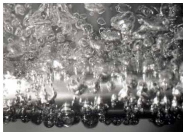
Fig. 12: The appearance of heat transfer surface during pool boiling of acetone ( q=380 kW/sqm).
