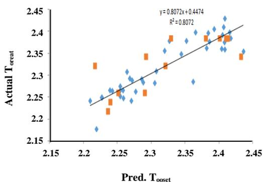
Figure 2: The plot of actual versus predicted of the training and test set's  $T_{onset}$  of the model I.
