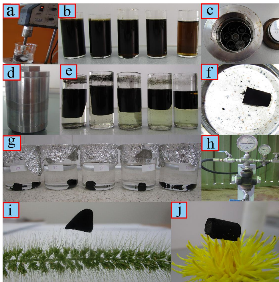
Fig. 2: Preparation procedure of GOPOS aerogels: ultrasonication process to disperse reagents in H 2 O/THF solvent (a), dispersed reactants in solvent media; left to right: GOPOS90, GOPOS70, GOPOS50, GOPOS30, GOPOS10 (b), reaction autoclave (c) and (d), assembled GOPOS gels; left to right: GOPOS90, GOPOS70, GOPOS50, GOPOS30, GOPOS10 (e), solvent exchange process (f) and (g), supercritical CO 2 dryer to convert gels to aerogels (h), digital photographs of flyweight GOPOS aerogels placed on top of a Hordeum marinum (i) and Taraxacum kok-saghyz (j).
