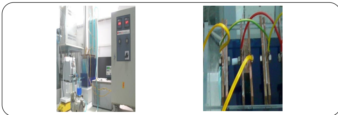
Fig. 3: Electrolytic refining process apparatus.
