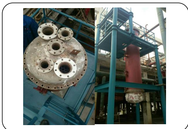
Fig. 4: Pictures of the multi-tubular fixed bed reactor for acetylene hydrochlorination.
