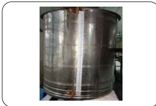
Fig. 1: Cylindrical tank with level indicator.
