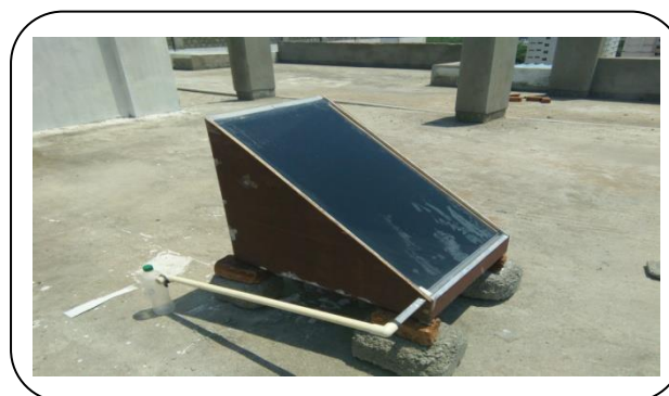
Fig.1: Solar Still Construction.
