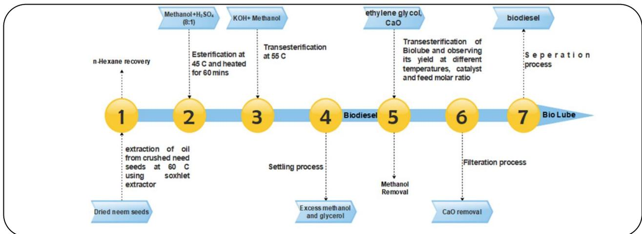
Fig. 2: Flow diagram for the synthesis of biolubricant from neem seed.
