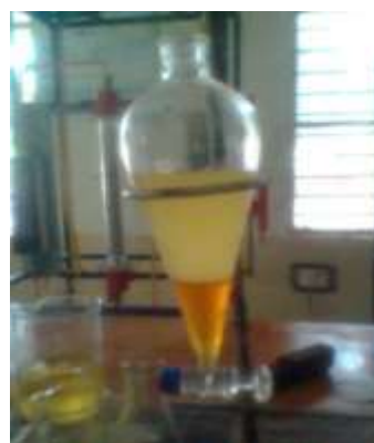
Fig. 5: Biodiesel separation from glycerol.
