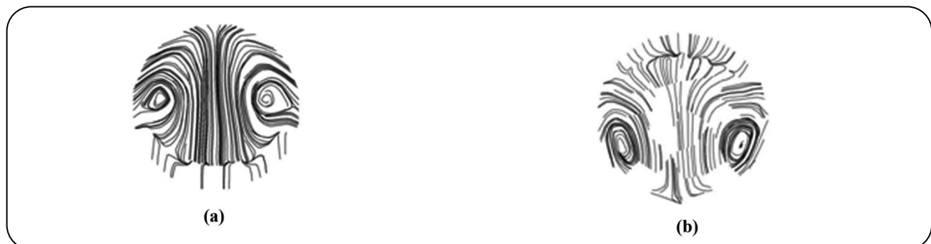
Fig. 15: (a) Secondary flow on the horizontal to vertical elbow's outlet cross-sectional plane. (b) Secondary flow on the pipeline outlet boundary, i.e., vertical to horizontal elbow.
